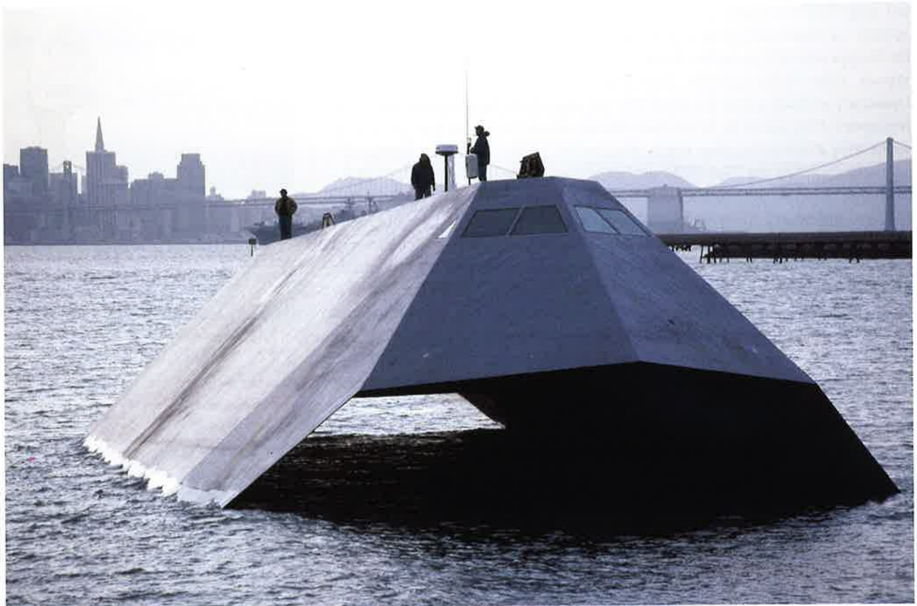
As shown in the photo on the previous page, Glosten designed the HMB barge/ floating drydock for the experimental stealth vessel SEA SHADOW (IX-529). She was designed and built by Lockheed for the United States Navy to determine how a low radar profile might be achieved, and to test high stability hull configurations which have been used in oceanographic ships. The SEA SHADOW had a SWATH hull design. Below the water were submerged twin hulls, each with a propeller, aft stabilizer, and inboard hydrofoil, and the superstructure above the water was connected to the hulls via the two angled struts. The SWATH design helped the ship remain stable in rough water up to Sea State 6, a wave height of 18 feet (5.5 m) or a very rough sea. In its aviation work, Lockheed also designed the U-2 and SR-71 Blackbird spy planes, and the F-117 Nighthawk stealth ground attack fighter.
