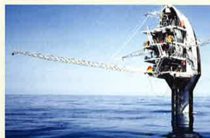
R/P FLIP (FLoating Instrument Platform) is an open ocean research platform owned by the U.S. Office of Naval Research (ONR) and operated by Scripps Institution of Oceanography. The platform is 108 meters (355 ft) long and is designed to partially flood and pitch backward 90 degrees, resulting in only the front 17 meters (55 ft) of the platform pointing up out of the water, with bulkheads becoming decks.
