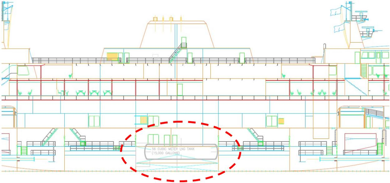
**Figure A3. 15,000 gallon LNG tank below EOS**
