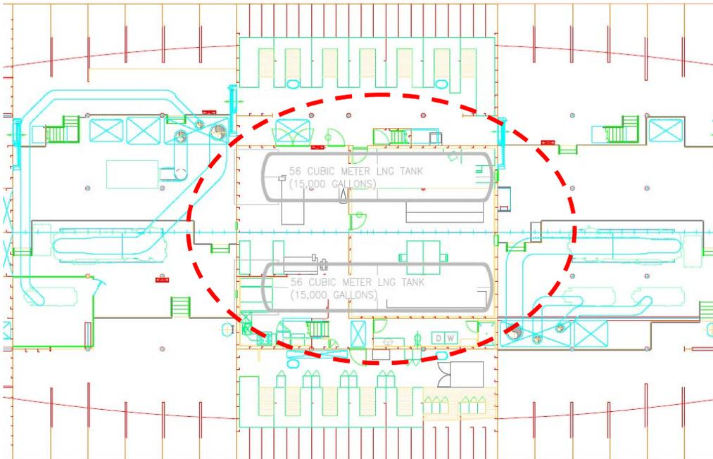
**Figure A4. Two 15,000 gallon LNG tank below EOS**
