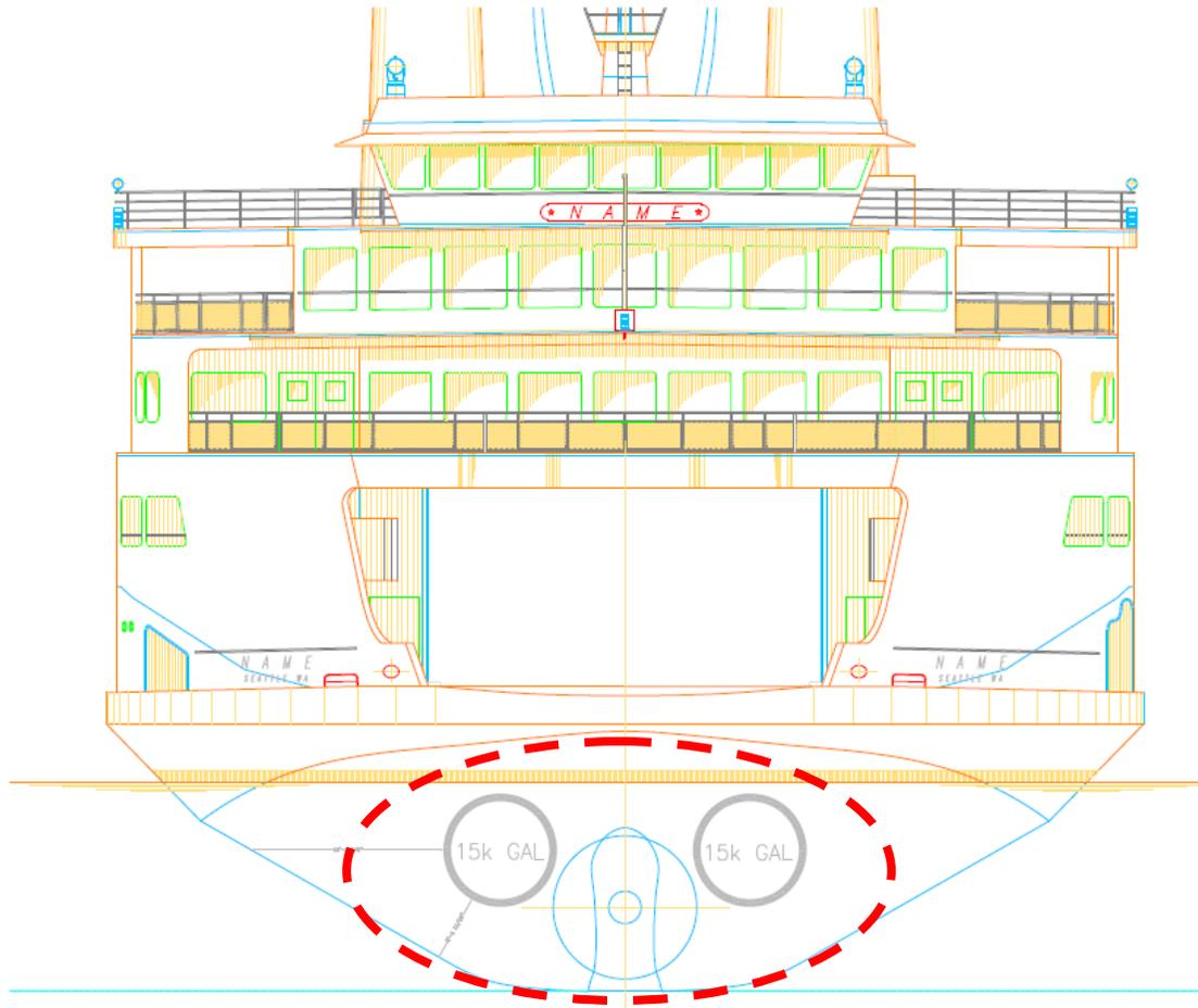
**Figure A5. LNG Tanks below EOS with minimum offsets from shell**
