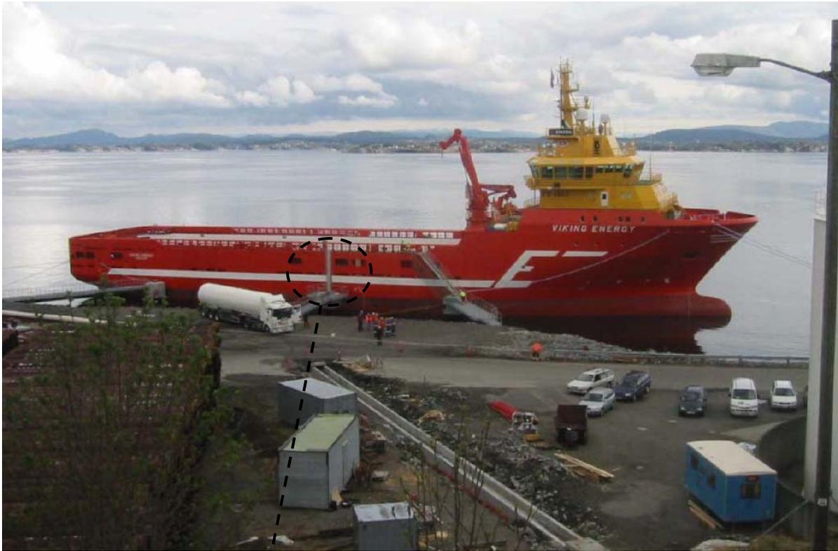
Figure A1, Quayside LNG bunkering with tank truck
