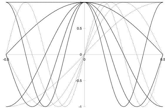
Fig. 4. Basis functions for sloshing modes; —, cosine; ·····, sine
