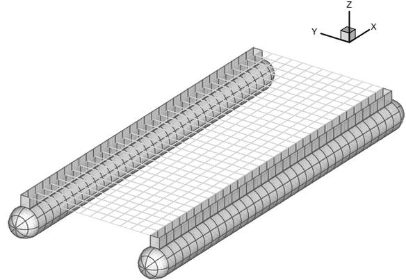
Fig. 3. Higher-order boundary element model showing panel subdivisions
