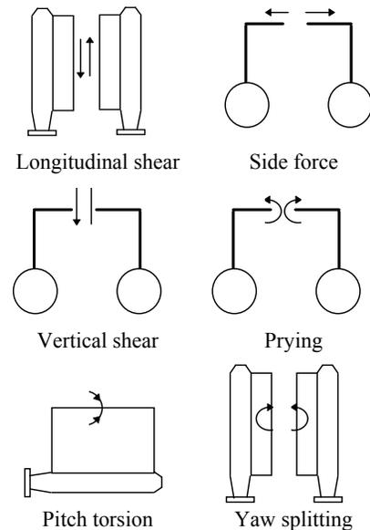
Fig 1. Differential loads for a SWATH vessel (ABS, 1999)
