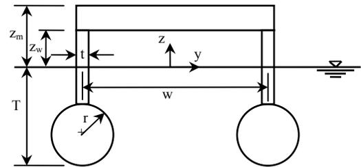
Fig. 2. Cross-sectional sketch of SWATH vessel
