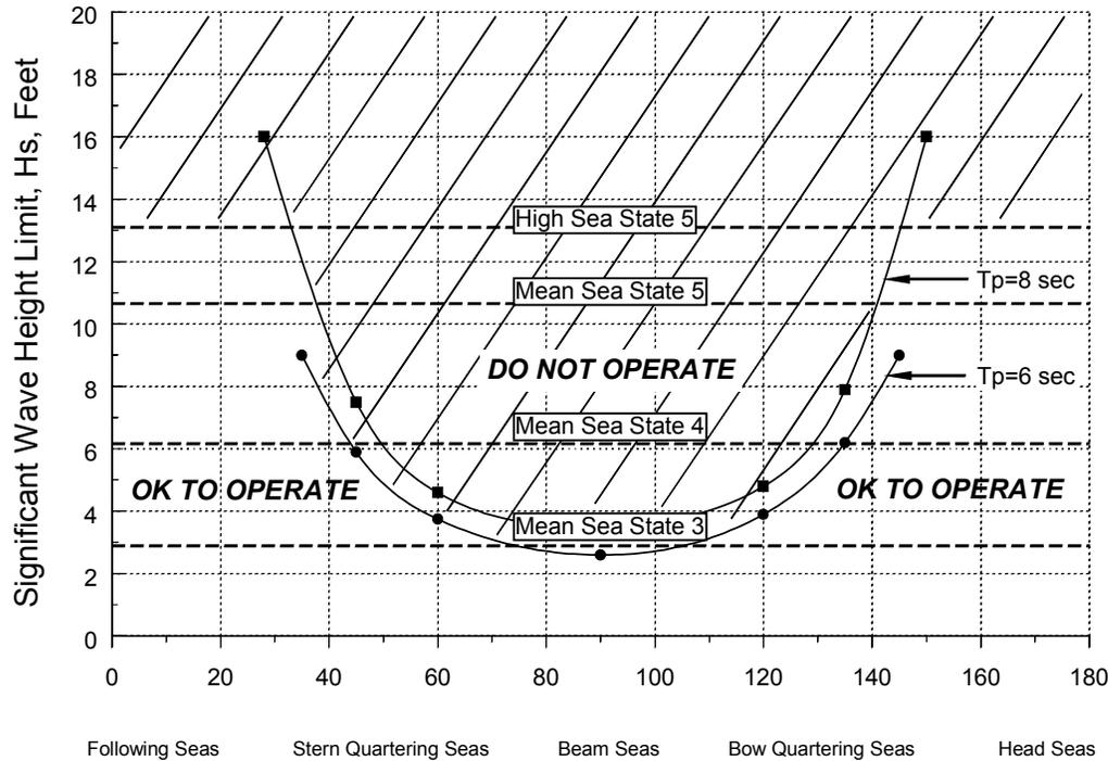
Figure 4. Operating Conditions in Various Wave Heights and Vessel Headings
