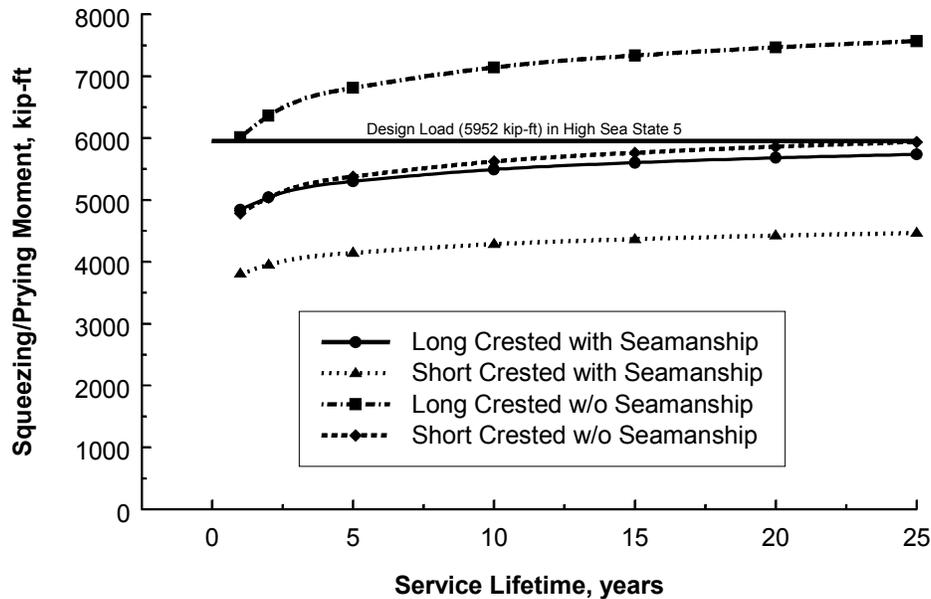
**Figure 6. R/V Western Flyer – Design Load, Existing Hull**
