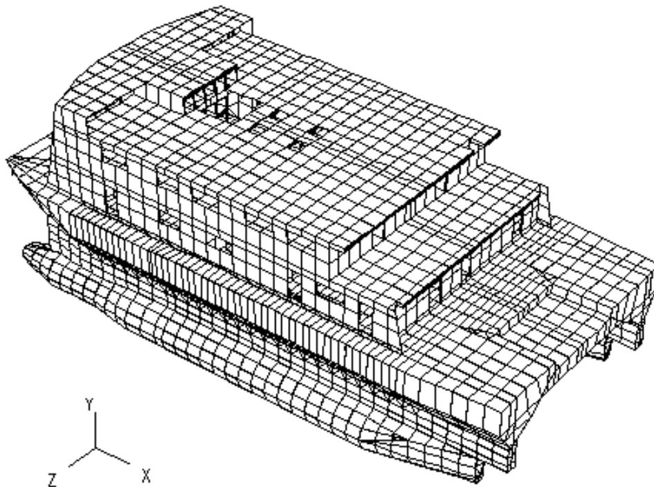
**Figure 5. R/V Western Flyer – Finite Element Model**
